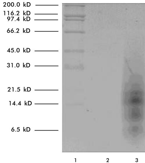
Figure 4. SDS-PAGE of the polymer under non-reducing conditions. The sample polymer was loaded onto the gel after extensive dialysis in a membrane of 6000–8000 molecular weight cut-off. Visualization was achieved by Coomassie Blue staining. Lane 1, molecular weight standards; lane 2, monomer peptide; lane 3, polymers. For unknown reasons, the band of the monomer peptide was not detected under standard conditions.
