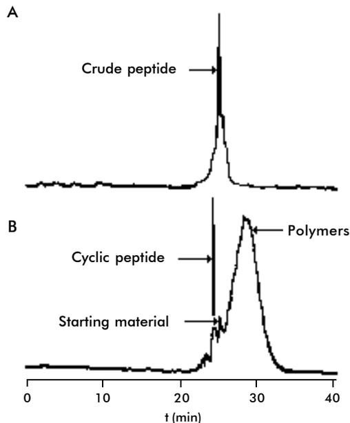
Figure 2. A) RP-HPLC using a Vydac C18 column of crude peptide C(Ac<sub>m</sub>)GRQSTPIGLGQALYTTKKQYIKANSKFIGITELGC(Ac<sub>m</sub>). B) HPLC of the crude peptide after stirring at room temperature for 30 min in AcOH/H<sub>2</sub>O (3:2) with 10 Eq of iodine. The arrows indicate cyclic peptide and polymer peaks.
