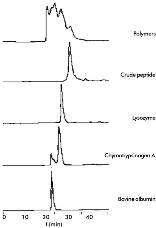
Figure 3. Gel filtration chromatography of peptide polymerization shown in Figure 2. The molecular weight standards shown are lysozyme, MW 14,000; chymotrypsinogen A, MW 25,000; and bovine albumin, MW 67,000. TSK G 2000SW column, equilibrated and eluted with 10% of acetonitrile, was used.
